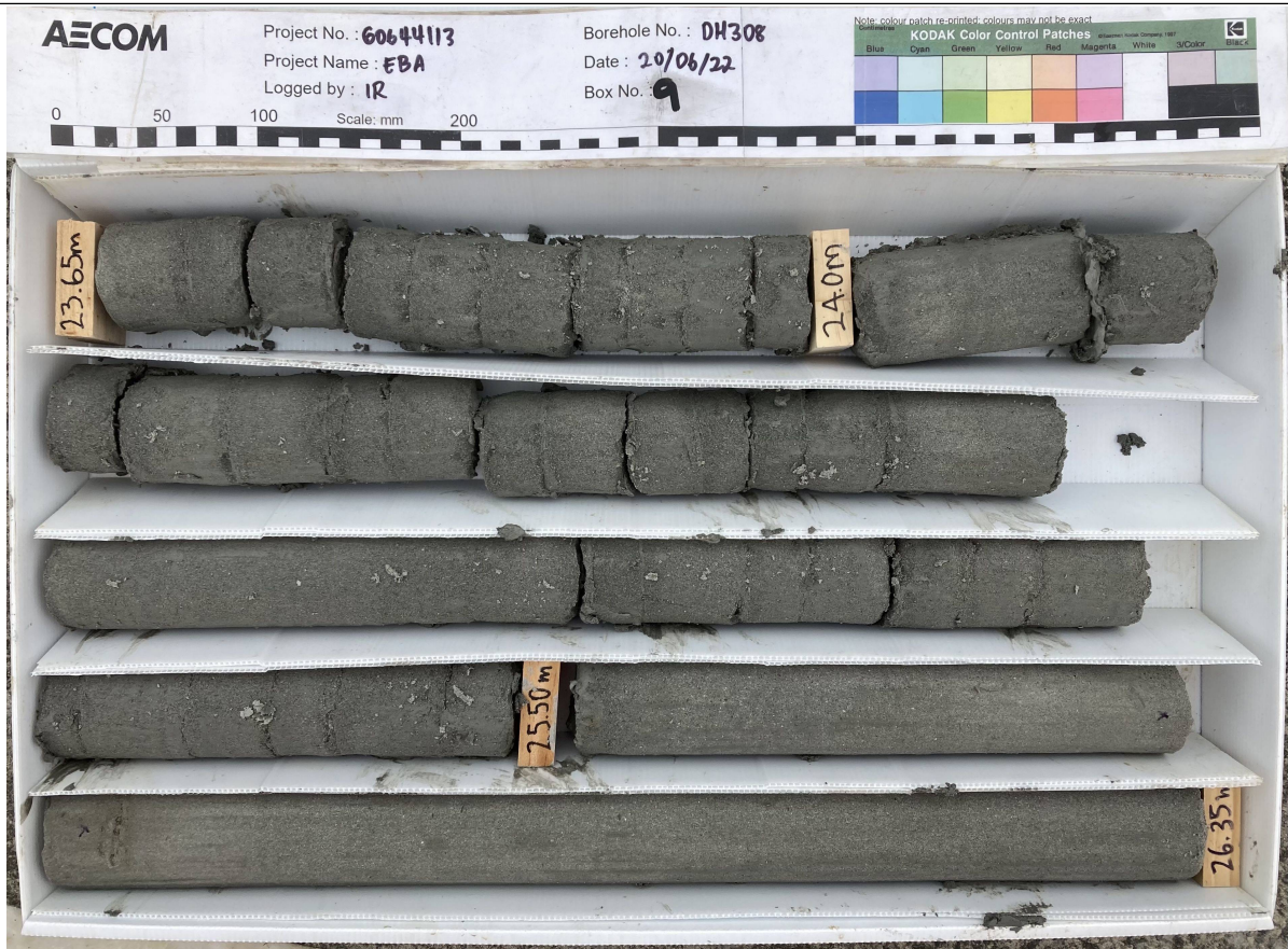
Box: 9 of 10 - Depth: 23.65m to 26.35m of 27.00m Date Drilled 17/06/2022 to 20/06/2022 - Date Photographed: 20/06/2022
